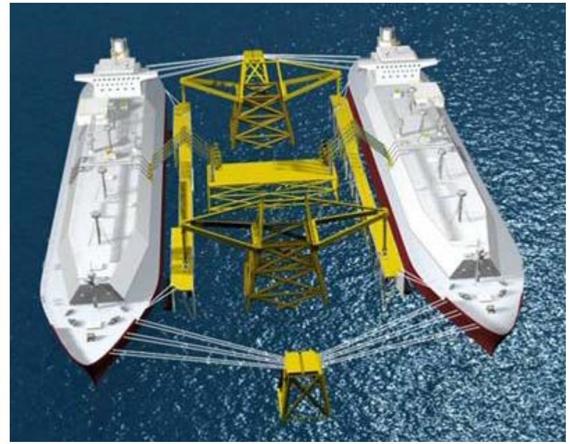
“TWIN SOFT QUAY MOORING”
