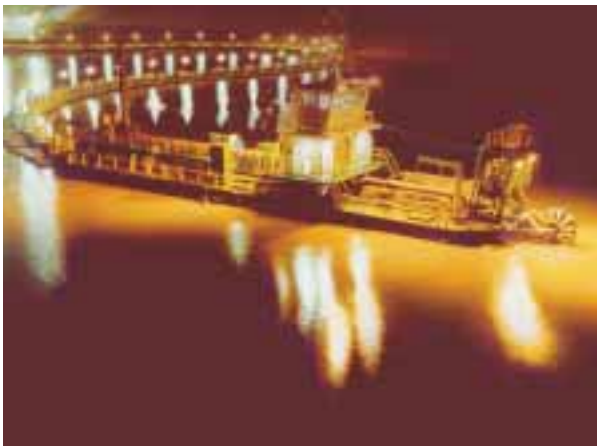
Heavy minerals wheel suction dredger for Millennium in Brazil.
