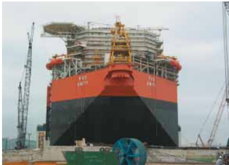
The FSO Unity, a turnkey supply for TotalFinaElf Nigeria. This VLCC size hull was assembled and outfitted onland in Hyundai and launched over the quay side – a unique method for such an operation.
