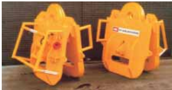
Chain clamps 500 ton for installation of mooring lines of the Spar 'Vastar Horn Mountain'.
