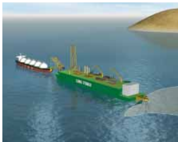
SBM's concept for a floating regasification plant (FSRU); an import terminal for liquefied natural gas.
