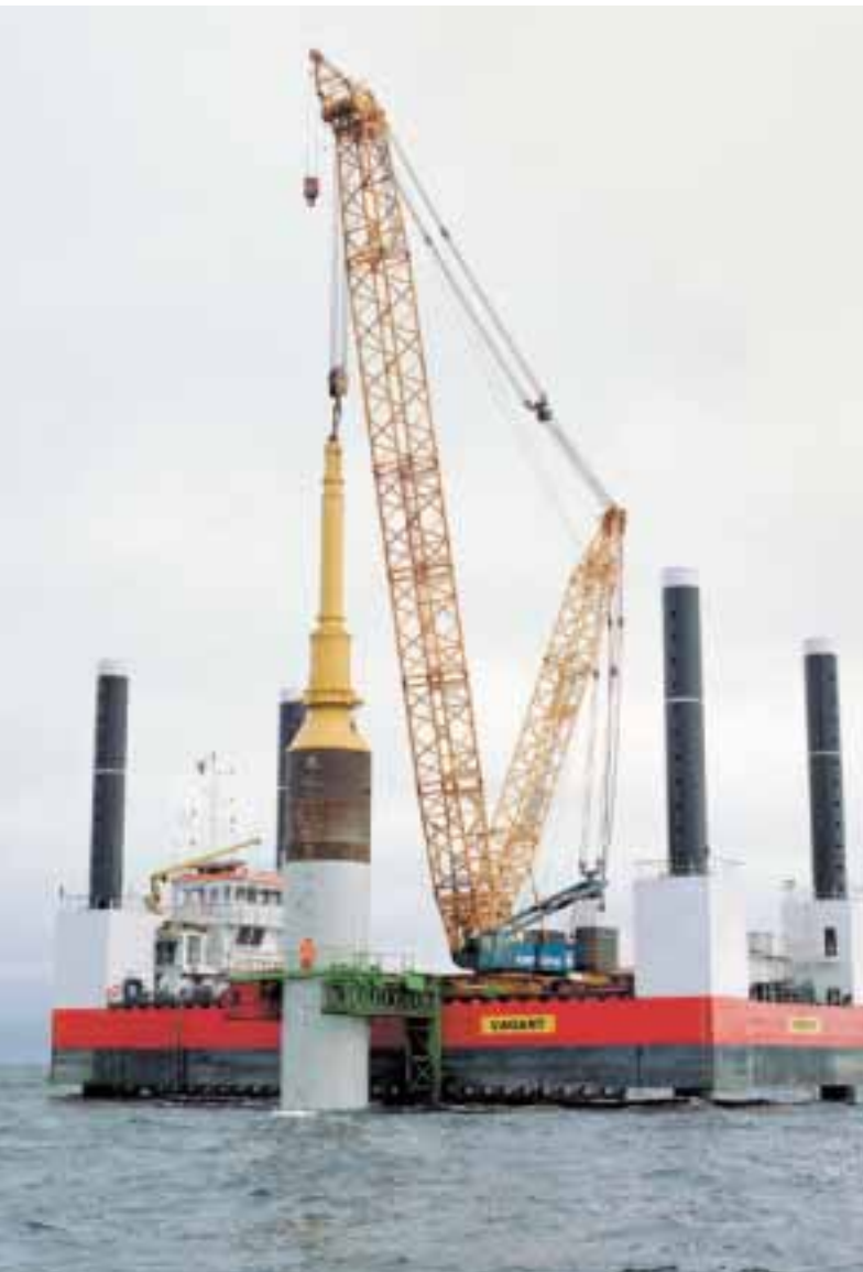
The MSC Sea800 jack-up Vagant for civil contractor HydroSoils, built by Merwede Shipyards.
