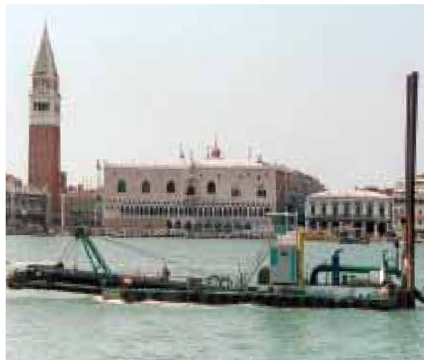
IHC cutter suction dredger type Beaver 1200 in Venice.
