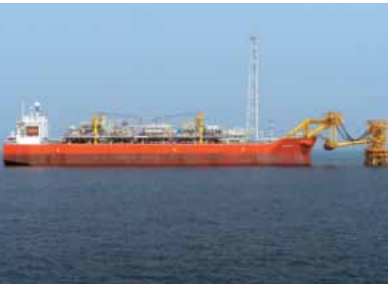
A view of the Shell EA FPSO connected to SBM's jacket/soft yoke system.
