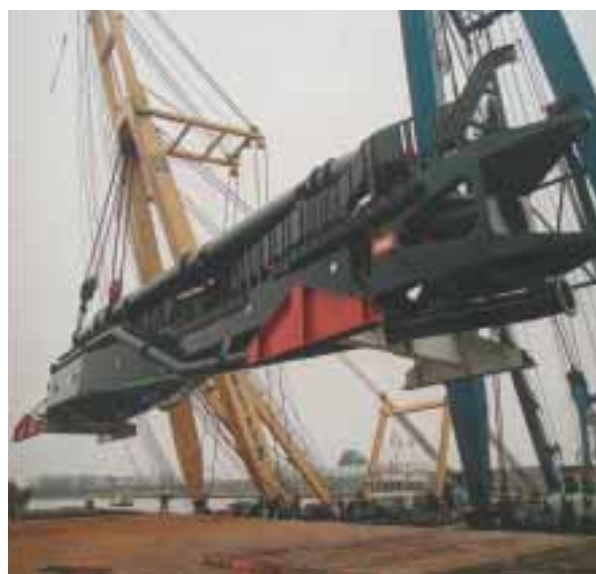
Transport of deepwater dredging installation for the 44000m 3 (after lengthening) trailing suction hopper dredger 'Vasco da Gama' for J. de Nul.
