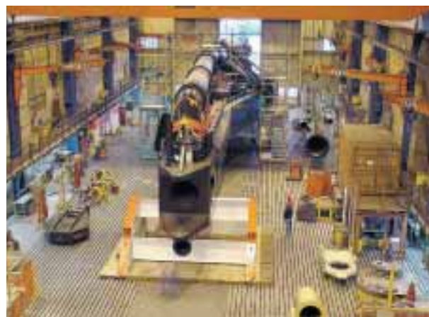
Deepwater dredging installation for the 44000m 3 (after lengthening) trailing suction hopper dredger 'Vasco da Gama' for J. de Nul.
