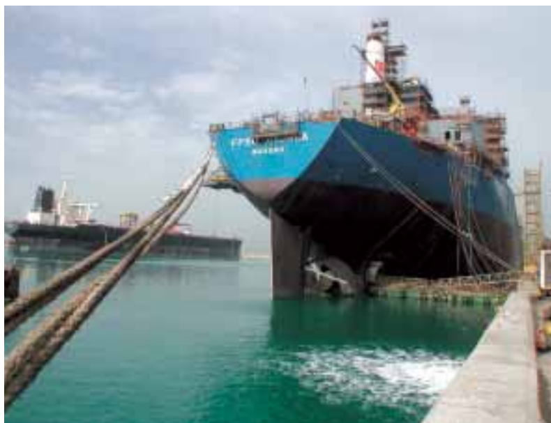
Xikomba FPSO, the third of the ExxonMobil Generic series, during conversion work alongside the quay in Dubai drydocks.
