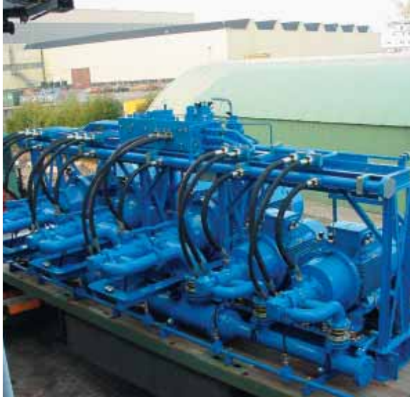
Hytop – 1500kW hydraulic powerpack
