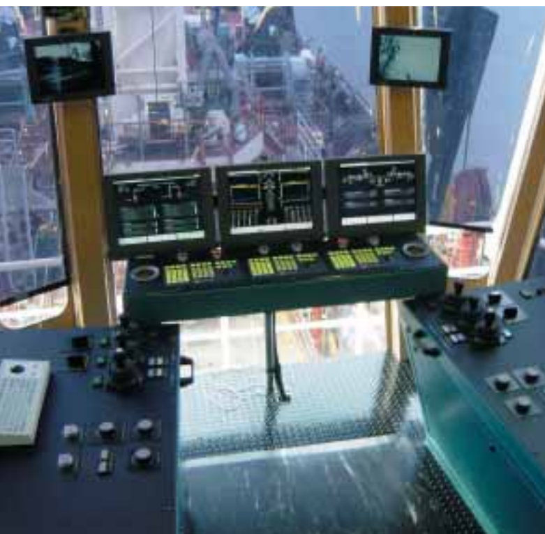
IHC Systems' Dredge Control Monitoring System (DCSM) on the trailing suction hopper dredger 'Essayons'
