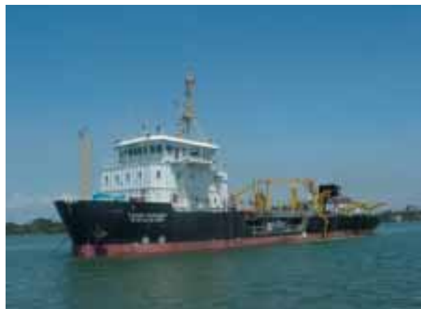
1700m 3 trailing suction hopper dredger for CPT, India
