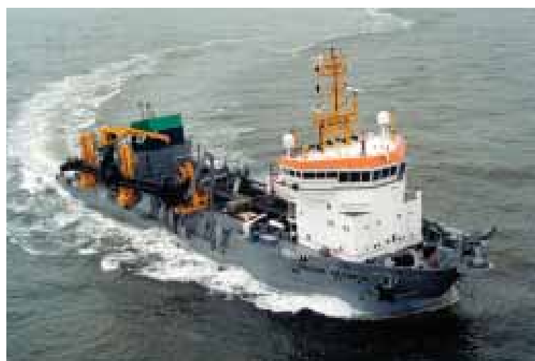
The 4750m 3 trailing suction hopper dredger 'Volvox Olympia'
