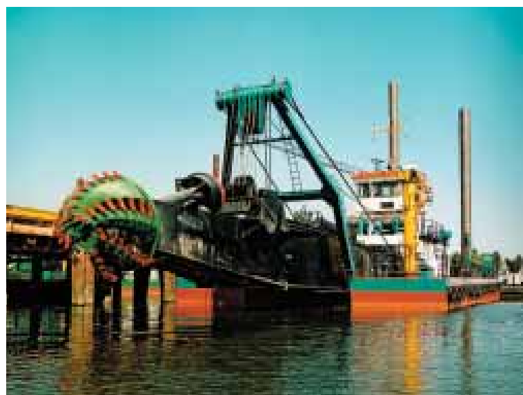
IHC Beaver cutter suction dredger equipped with an IHC cutter for Nigeria
