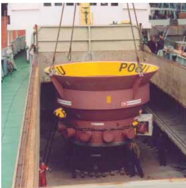
IHC Handling Systems – 2500tons pile gripper
