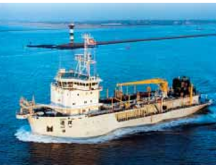
The 3500m 3 trailing suction hopper dredger 'Tong Tan' for China
