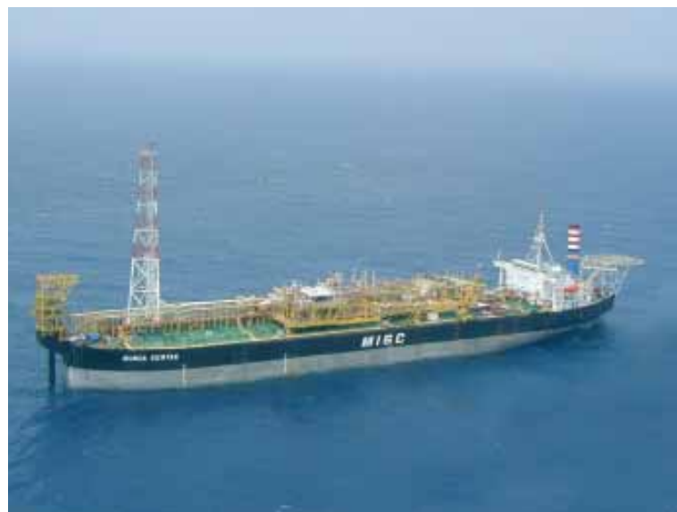
The Bunga Kentas FPSO for MISC (Malaysia), moored by an external turret delivered by SBM group
