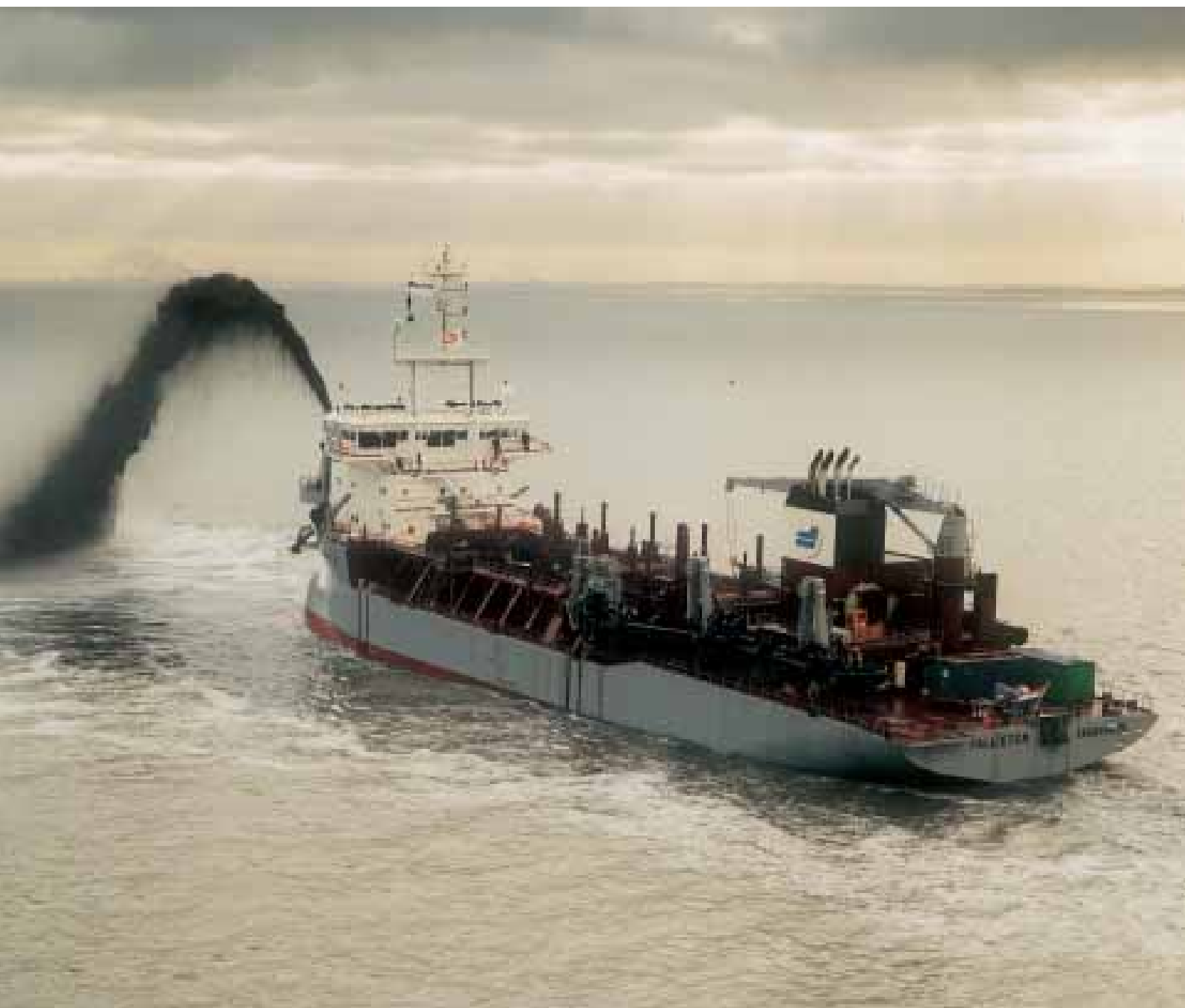
The 5400m 3 suction hopper dredger 'Pallietier' for DEME, Belgium
