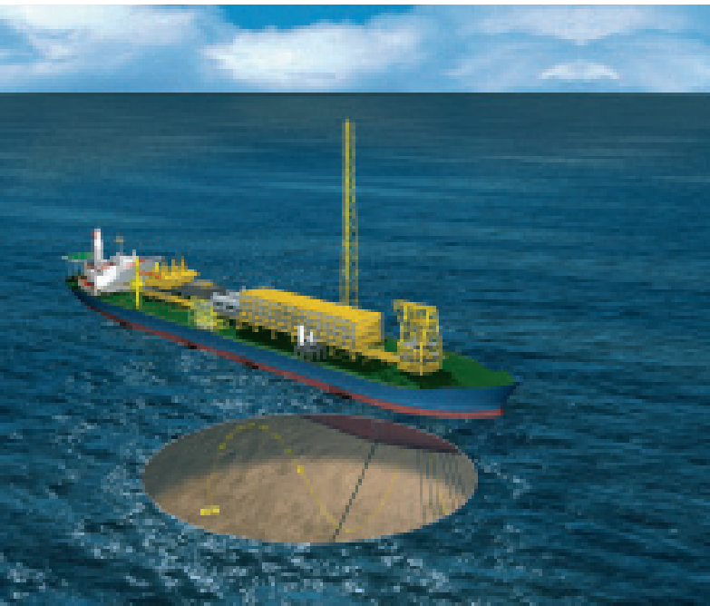
An FRU for receipt and regasification of LNG and subsequent storage of gas in subterranean salt caverns
