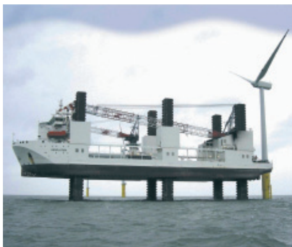
The windmill installation vessel 'Resolution'
