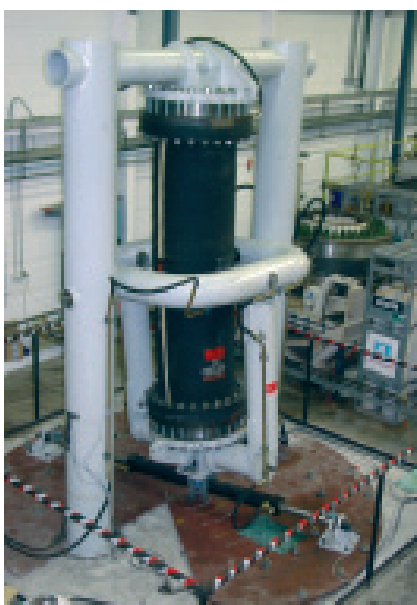
Full scale fatigue test of the Trelline Gimbal hose in SBM's testing facilities
