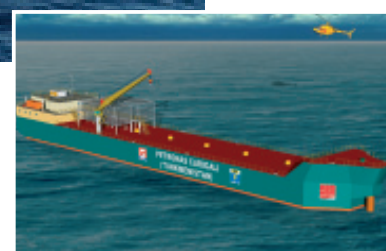
The two components of the EWT offshore Turkmenistan: a Mobile Offshore Production Unit and an FSO
