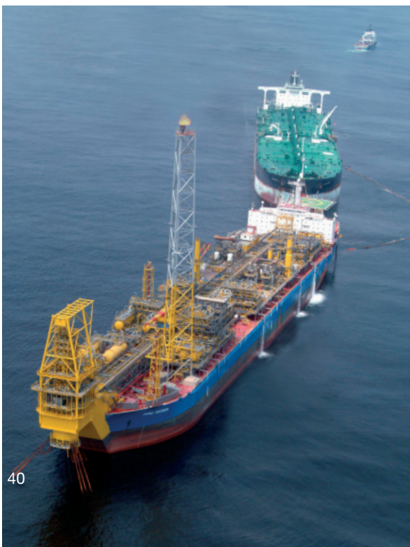
The FPSO Xikomba during an offloading operation
