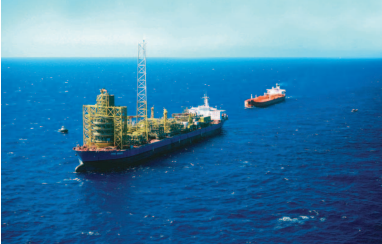
FPSO Brasil during an offloading operation transferring cargo to an export tanker
