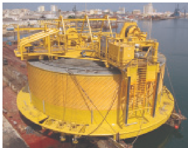
The Kizomba A deepwater export buoy ready for launching at the Sonamet yard in Angola
