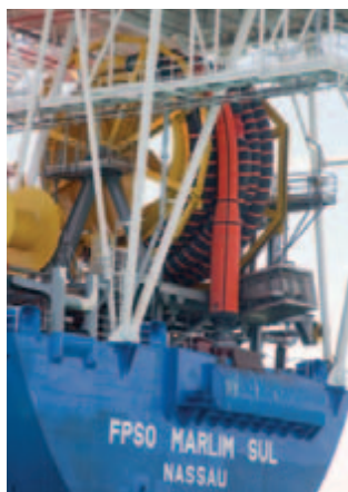
The offloading hose reel of the FPSO Marlim Sul designed and supplied by Gusto
