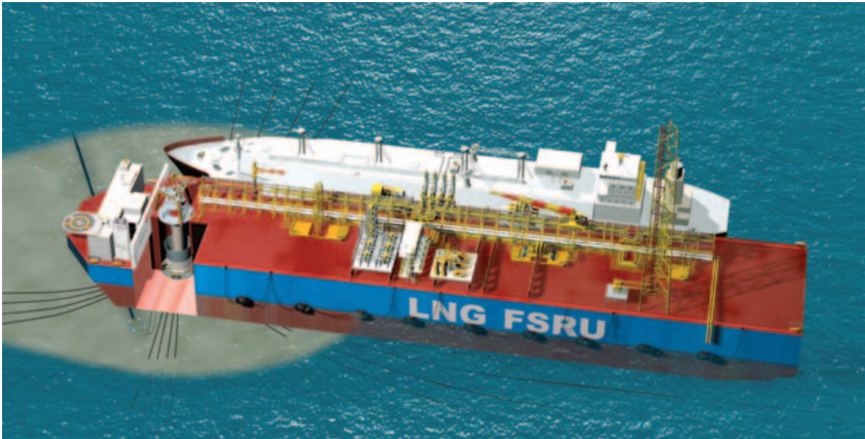
A large new build FSRU, moored by an internal turret, with an LNG carrier discharging cargo moored alongside
