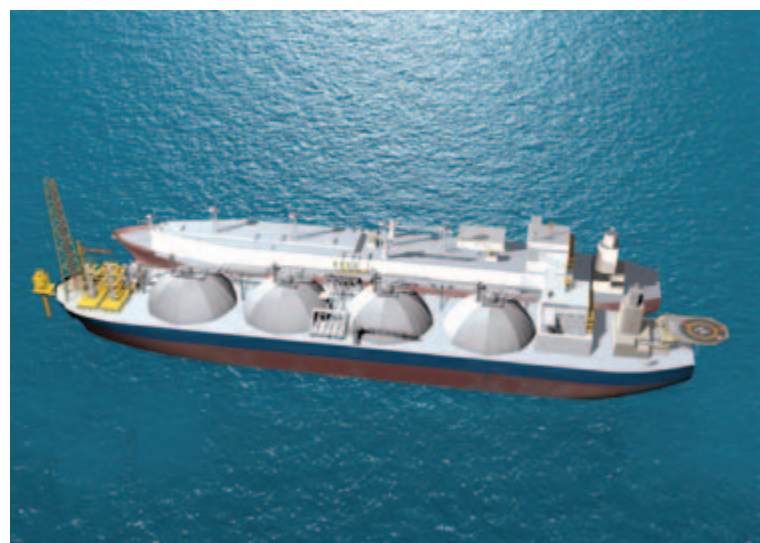
A small FSRU converted from a LNG carrier moored by an external turret
