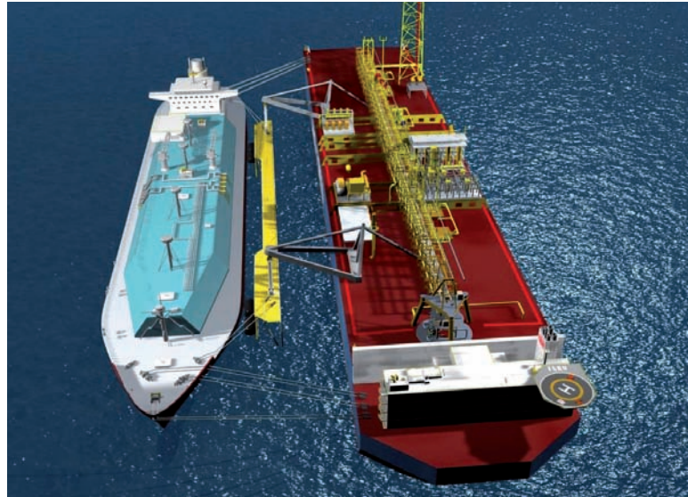
A 'Soft Quay Mooring' allows offloading of an LNG carrier into an FSRU at high sea states
