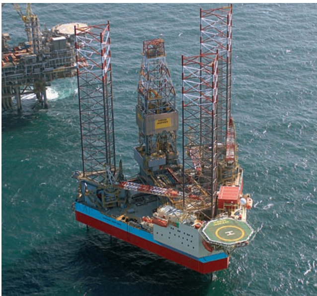
Jack-up 'Maersk Inspirer' converted into a drilling and production unit for the Volve field
