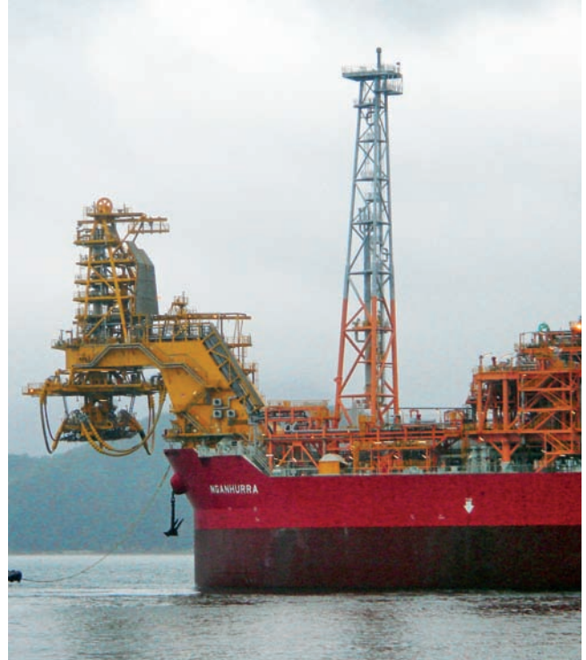
Cantilever structure at the bow of the Enfield FPSO comprising the manifolding and swivel arrangement of the disconnectable turret
