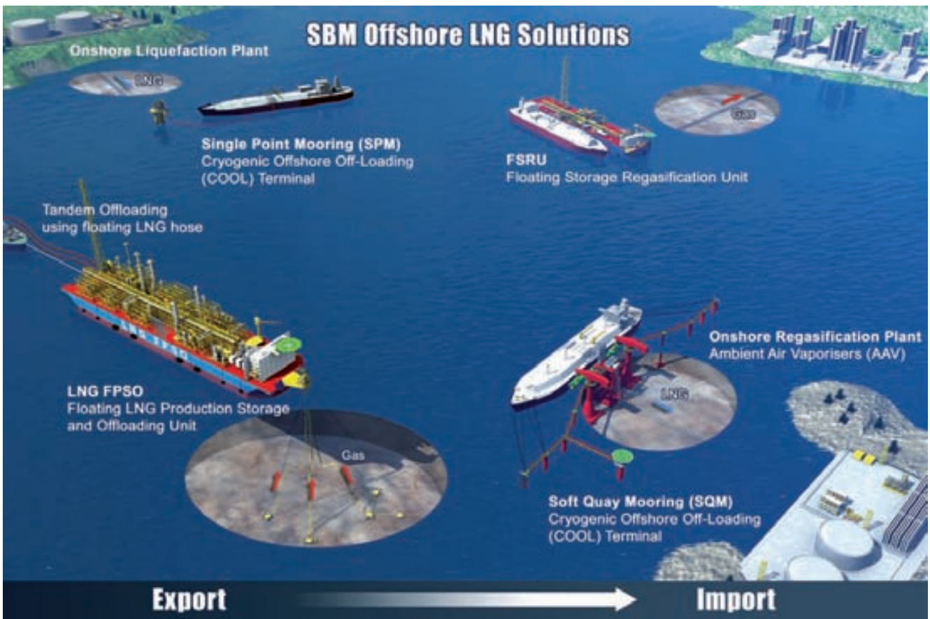
SBM Offshore solutions for export, import and offshore production of LNG
