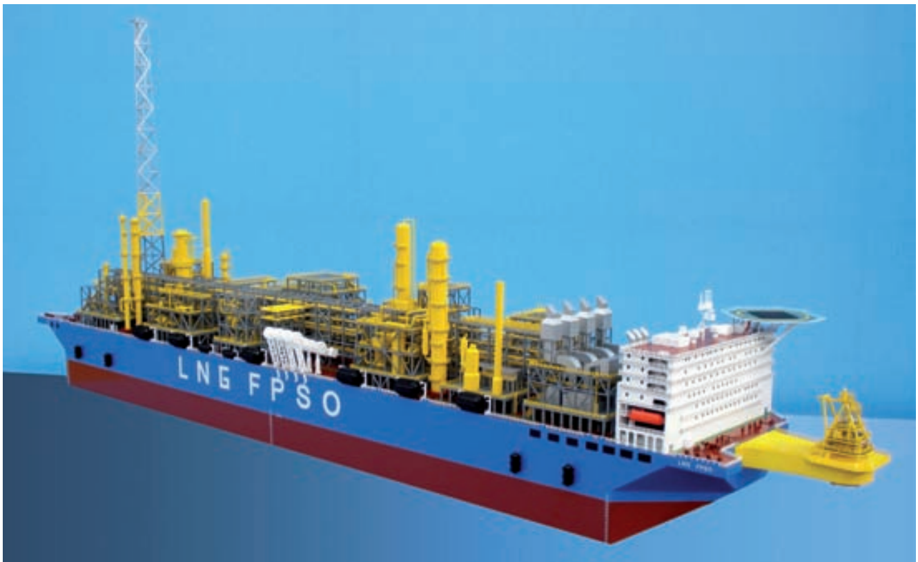
SBM-Linde's design for processing, liquefaction, storage and offloading of LNG and associated products from offshore stranded gas fields
