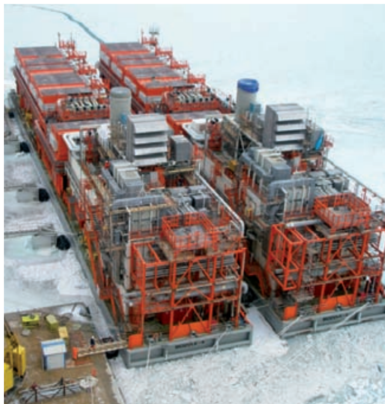
Flash gas compression Barges 3 and 4 at Kuryk, Kashagan, Caspian Sea prior to offshore installation
