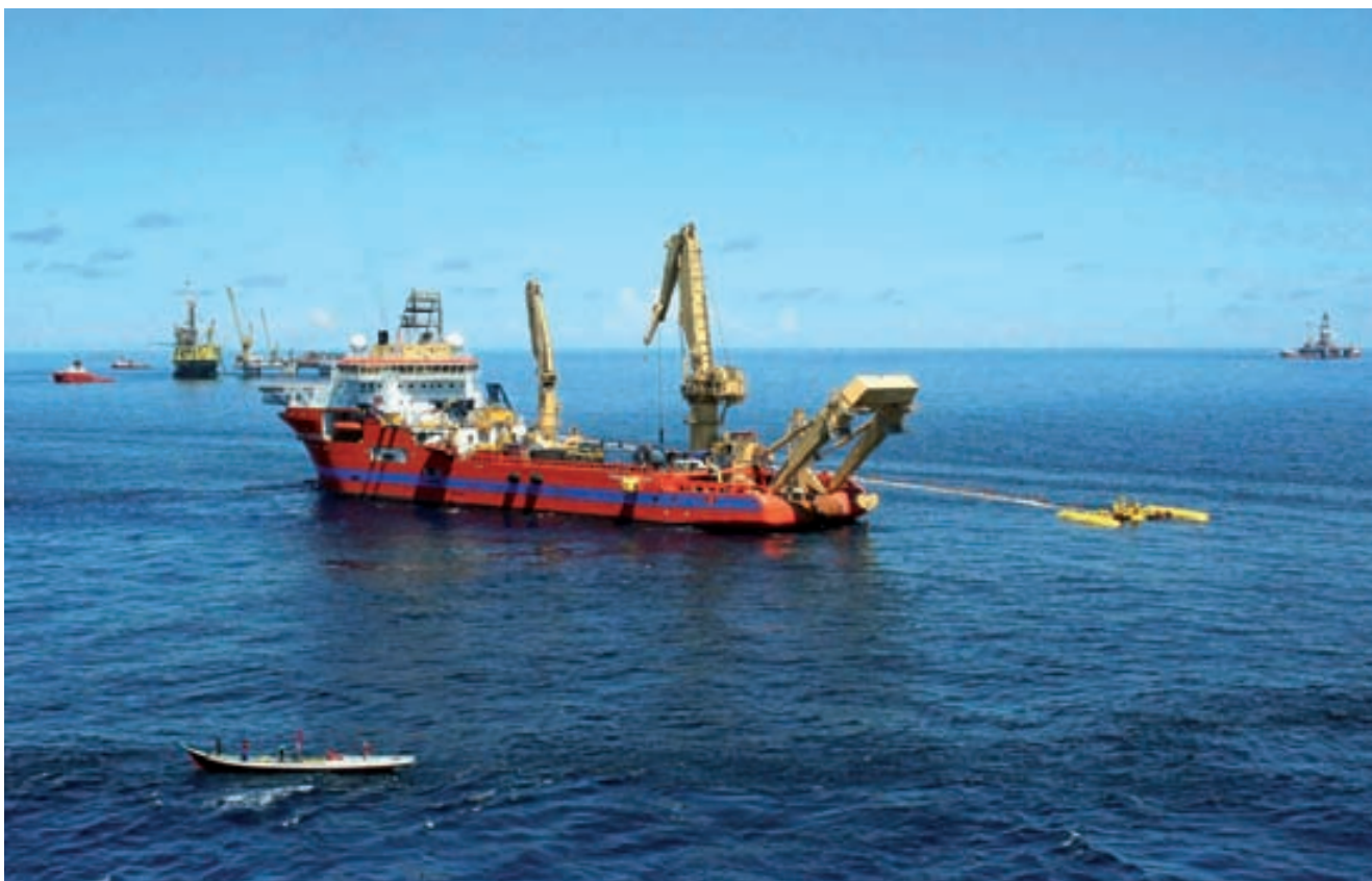
Normand Installer towing the GAP™ on the Kikeh Field, Malaysia
