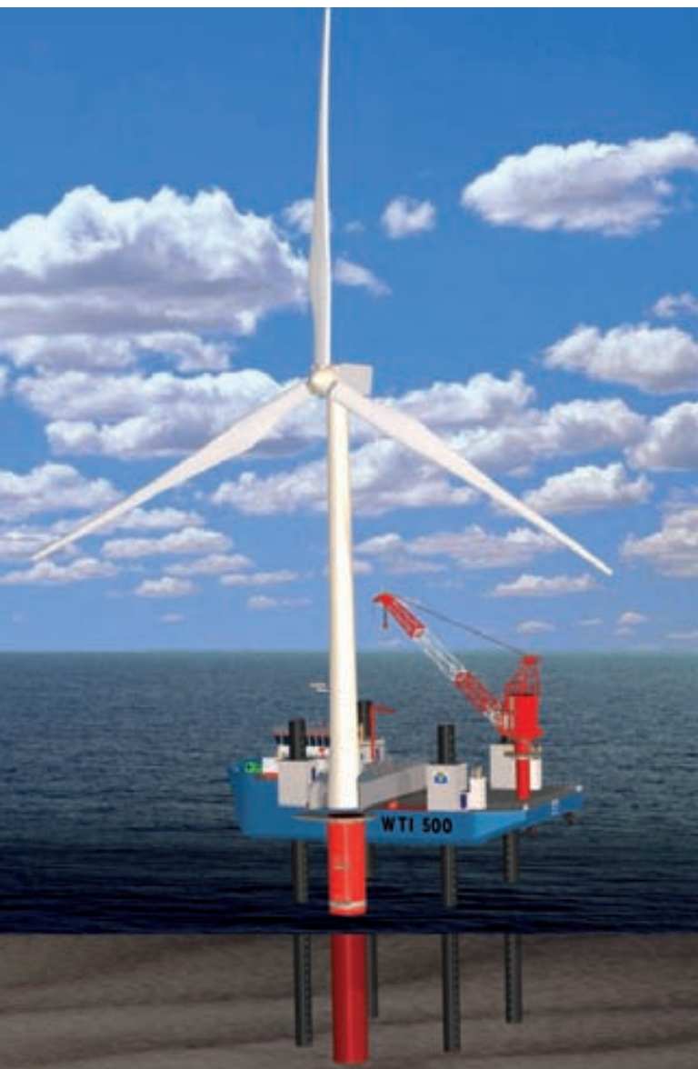
Wind Turbine Installation Jack Up, designed by GustoMSC
