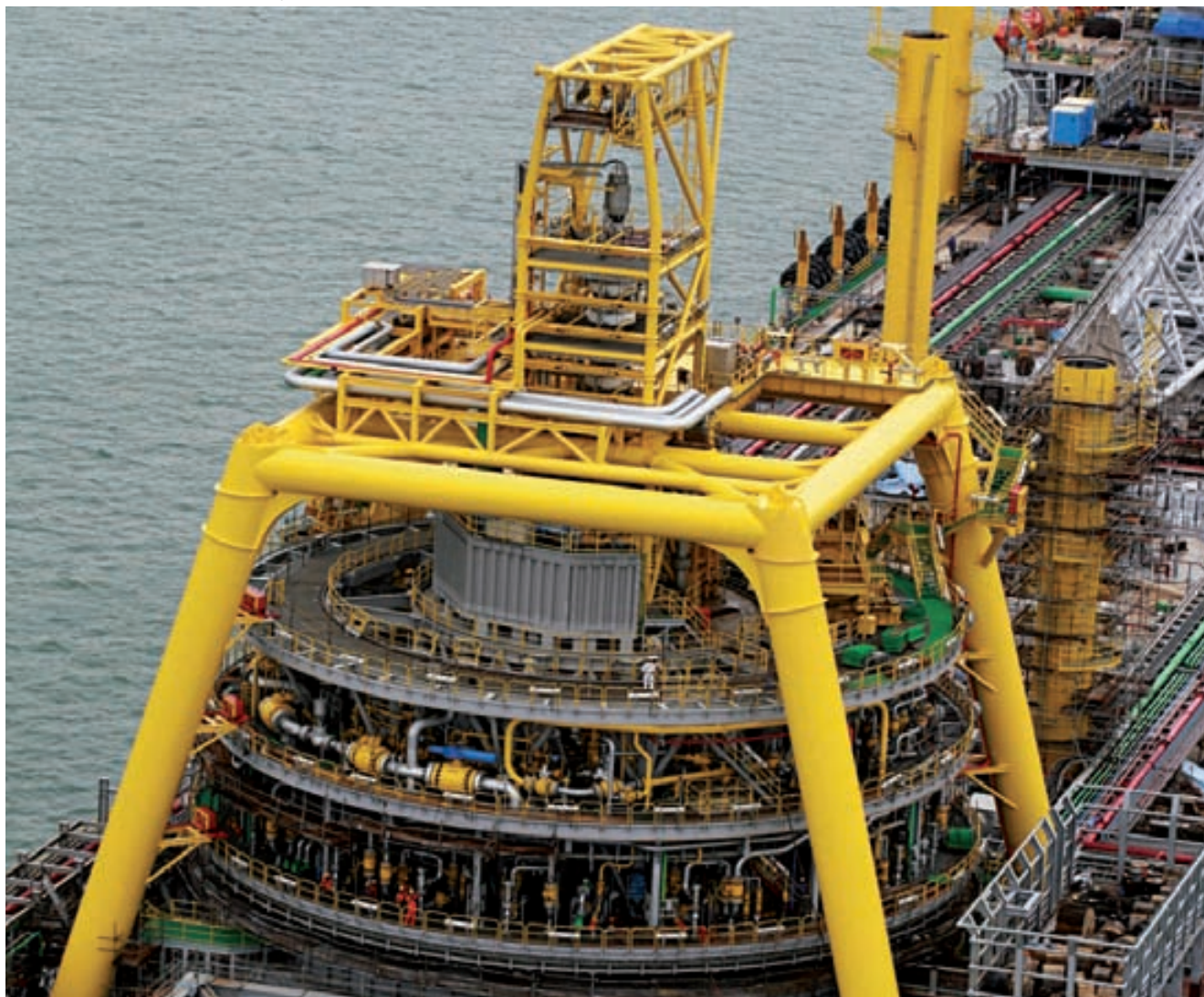
Petrobras P53 turret, the world largest with 75 riser slots
