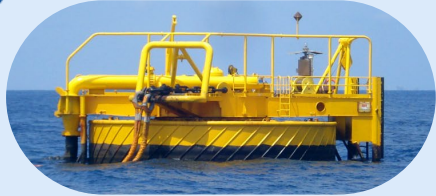
Ammonia CALM terminal
